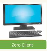
Essentially, zero clients are minimalistic computers relying on a server to manage functions that a traditional PC (thick client) would handle with its own hardware and software. Primarily employed in virtual desktop infrastructure (VDI) setups, zero clients excel in remote work scenarios or distributed work environments.
